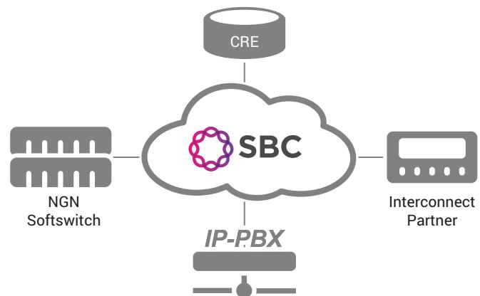
existing legacy NGN infrastructure to interconnect with the PTT in compliance with the SIP Interconnect specifications. The advanced SBC includes onboard transcoding capabilities to address the interworking between voice solutions, an ongoing limitation of the customer's network.
